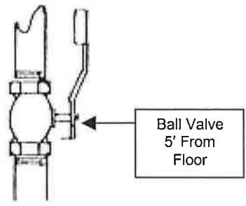
**NOTE: STATE APPROVED PRESSURE REDUCER DEVICE REQUIRED AT 80 PSI AND GREATER. PRESSURE REDUCING VALVE MUST BE INSTALLED AFTER THE METER. COPPER SWEAT FITTINGS CAN BE SUBSTITUTED FOR BRASS.**
