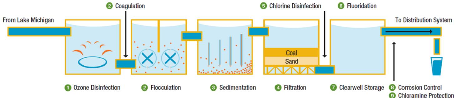
**(1) Ozone disinfection:** Ozone gas is bubbled through the incoming lake water. Ozone destroys disease-causing microorganisms including *Giardia* and *Cryptosporidium*, controls taste and odor, and reduces the formation of chlorinated disinfection byproducts.
