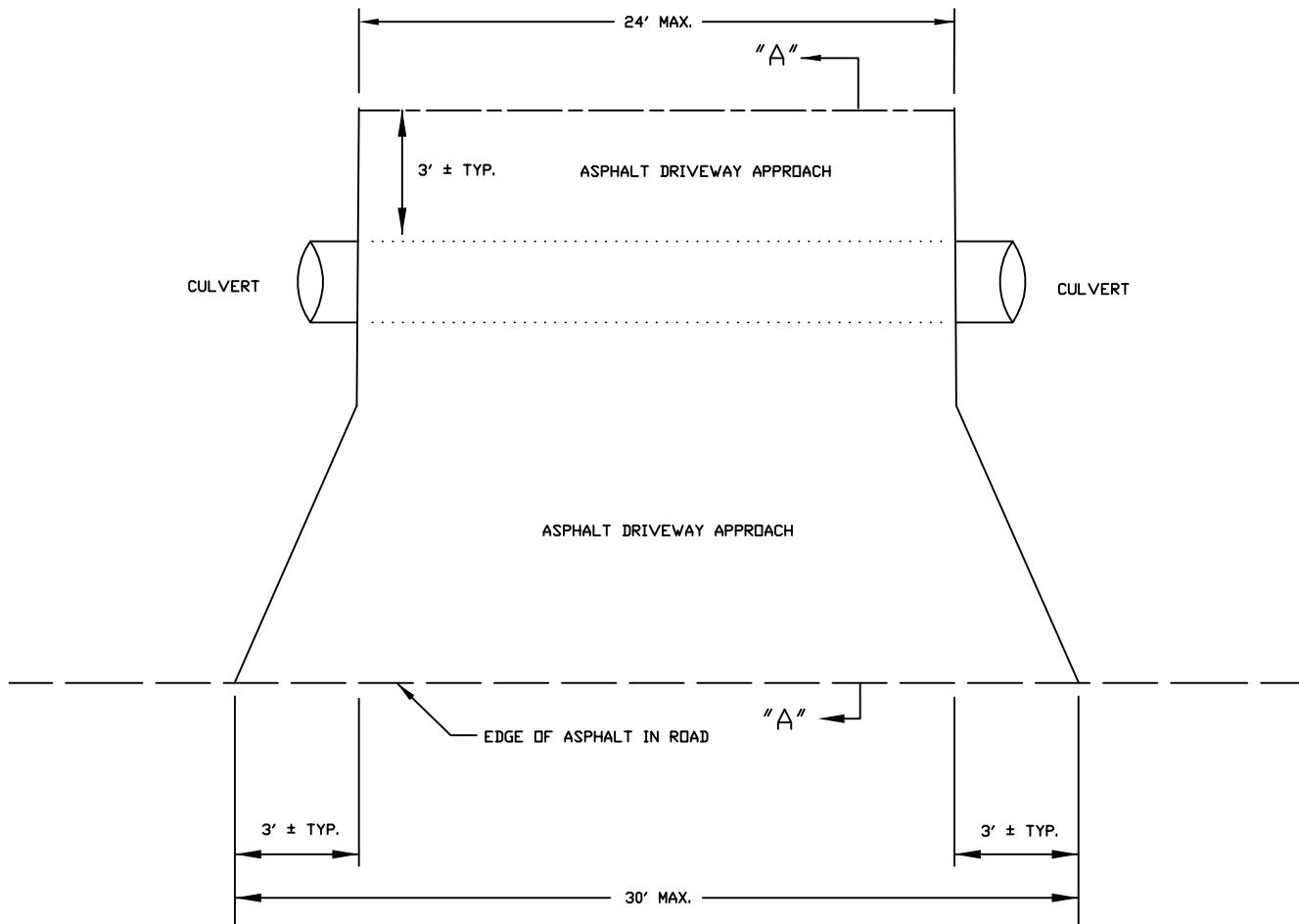
SUBGRADE NOTES: CONCRETE - 4" MINIMUM THICKNESS OF WELL COMPAKTED 3/4" CRUSHED LIMESTONE BASE COURSE REQUIRED UNDER DRIVEWAY APPROACH.
