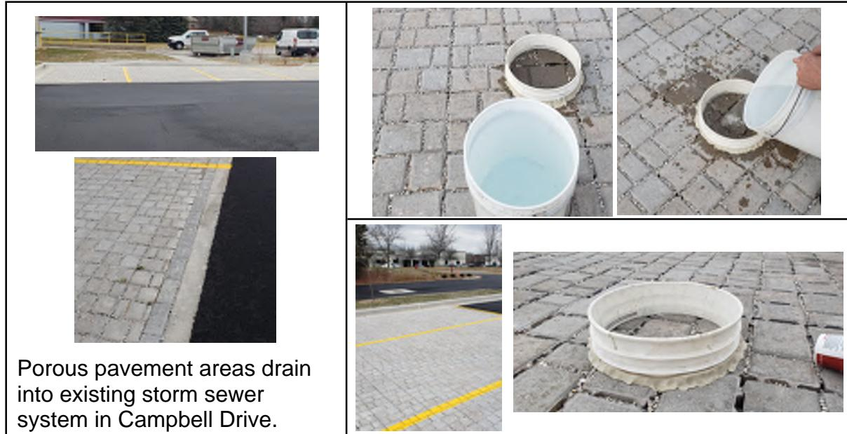
Porous pavement areas drain into existing storm sewer system in Campbell Drive.
