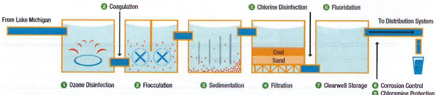
**(1) Ozone disinfection:** Ozone gas is bubbled through the incoming lake water. Ozone destroys disease-causing microorganisms including *Giardia* and *Cryptosporidium*, controls taste and odor, and reduces the formation of chlorinated disinfection byproducts.
